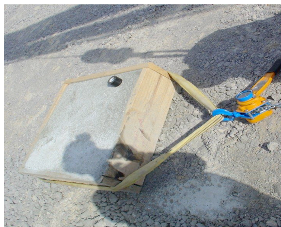
Figure 2.5.1: Concrete Test Block on Crushed Rock
