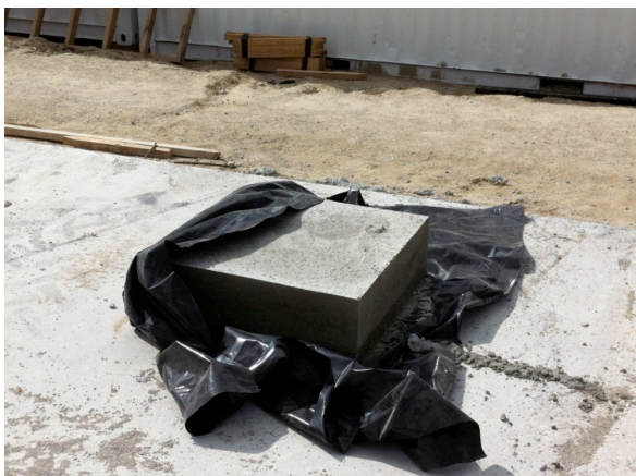
Figure 2.5.2: Test Block on Polyethylene
